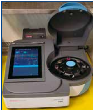
Figure 2B. Quantitative photometric measurement of coloured solution based on the reaction of urine PBG with Erlich reagent.
