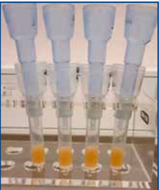
Figure 2A. Processing of urine before the Erlich reaction by solid phase extraction and separation on an anion-exchange column.
